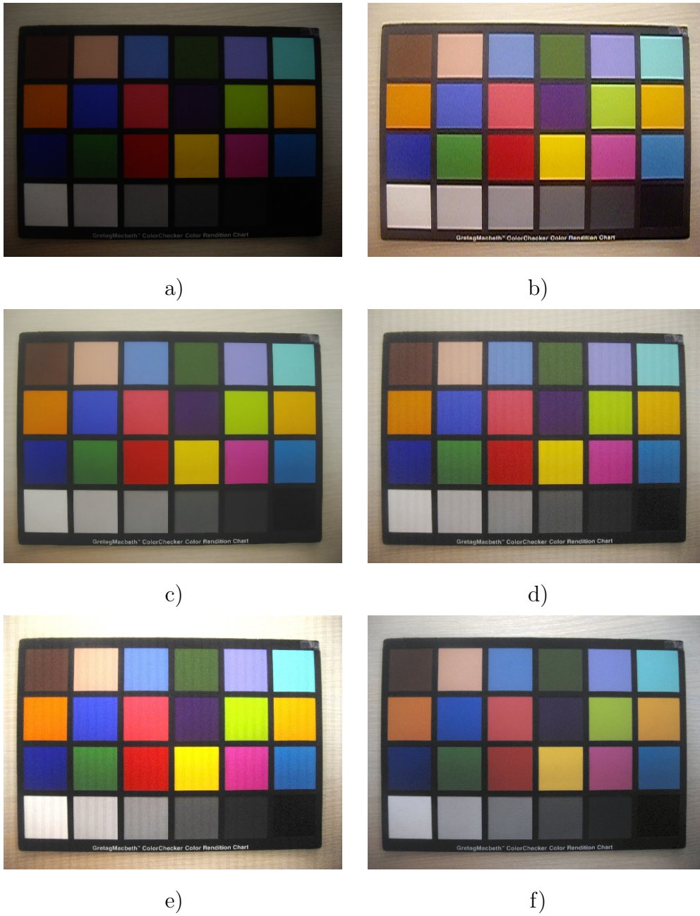
Figure 4.1: (a) Under-exposed subject image; (b) Motion blur-degraded reference image; (c) Ideal image; (d) Logarithmic amplified image; (e) Linear amplified image; (f) Auto-Contrast Image.
