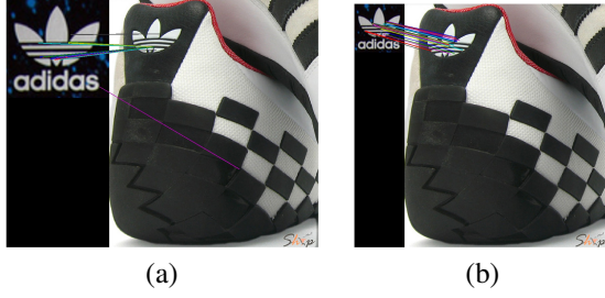
Figure 11. (a) The failed detection of the very small logo. (b) The successful detection after resizing the test image.
