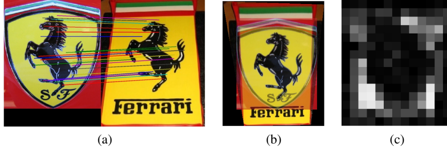
Figure 7. Constructing the error map (a) The matching pairs of points (b) The mosaic of images after applying the found homography. (c) The error map. The darker areas show good quality of matching.
