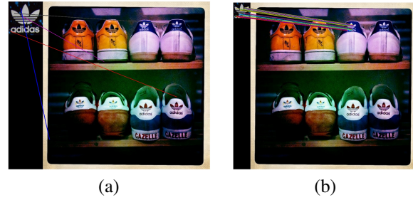
Figure 8. (a) Matching fails when using only the central image. (b) Successful detection when using the model of the class. We note that, for clarity, only the first detection is showed in the right hand plot, while in this case all Adidas logos were, in fact, found.
