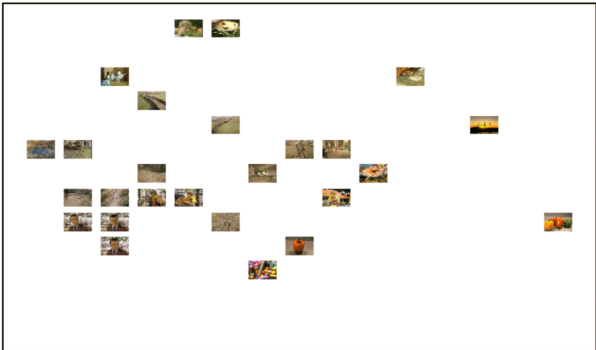
Fig. 3: Two-dimensional image scatter-plot of images within the database, according to the similarity relations between the images and the image at the center. The distances within the image locations are proportional to the image similarity.
