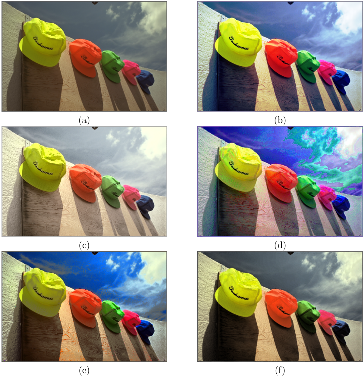
Figure 3: Results of histogram equalization: (a) The original 256 \times 384 pixel “03” image. (b) The image after histogram equalization on each channel independently. (c) The image after 3-D histogram equalization. (d) The image after histogram decimation. (e) The image after histogram explosion. (f) The image after ANHE with N_{max} = 100 , N_{min} = 20 , T = 20 , and \kappa = 3 .
