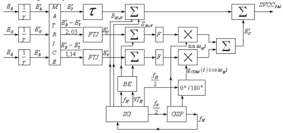
There are two processing paths in this diagram: the luminance and the chrominance path, as defined by the signals that it processes. Input signals are the three primary color signals received from the optoelectronic transmitter (camera), and has the following scheme.
