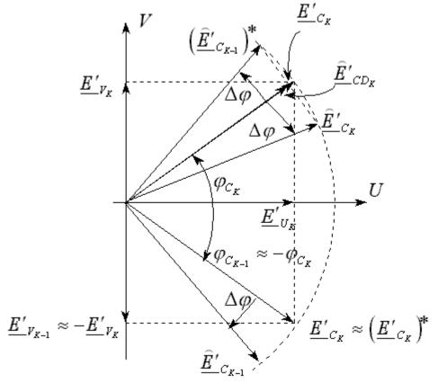
The chrominance signal on line K is represented by the vector  $\underline{E'}_{C_K}$ . The polarity of  $E'_V$  is changed from one line to another. At the reception, if there is a phase error, the vector will be  $\underline{\widehat{E'}}_{C_K}$ , with phase error  $-\Delta \varphi$ . The average value of vector  $\underline{\widehat{E'}}_{C_K}$  (chrominance signal on line K)
